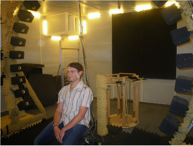
Figure 1: HRTF measurement setup at the Acoustics Research Institute, Austrian Academy of Sciences, Vienna.
